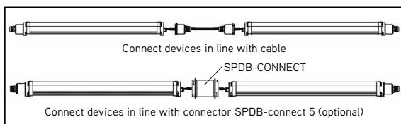
Speedy Basic can be easily connected using the SPDB-CONNECT coupling piece (to be ordered separately).
