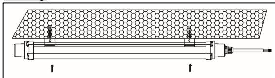
Drill two 6mm holes in the ceiling/wall where you want to install the fixture. The distance between the mounting brackets is freely selectable. Mount the mounting brackets with the supplied screws and plugs. Snap the fixture into the mounting brackets by pushing it into the mounting clips. Make sure the clips snap into place. If desired, the mounting brackets can be firmly anchored with the supplied bolts M4x60 + nut.
